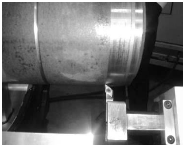
SEAL AREA BEING MACHINED TO N9 FINISH.
